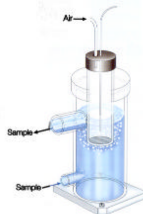
Figure 2. The New Backwash Strainer Unit
